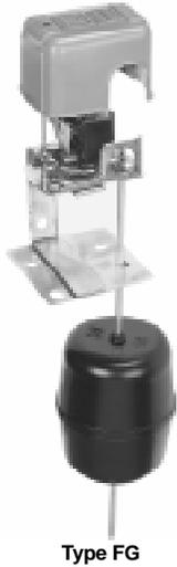
The Class 9036 Type FG30 pedestal style sump pump switch is designed for liquid level control with electric motor operated pumps either directly or through a magnetic starter. It can also be used to activate alarms in liquid level control systems. The upward or downward movement of the lever arm controls the ON and OFF positions corresponding to the water level changes required to turn the pump or alarm on and off.
